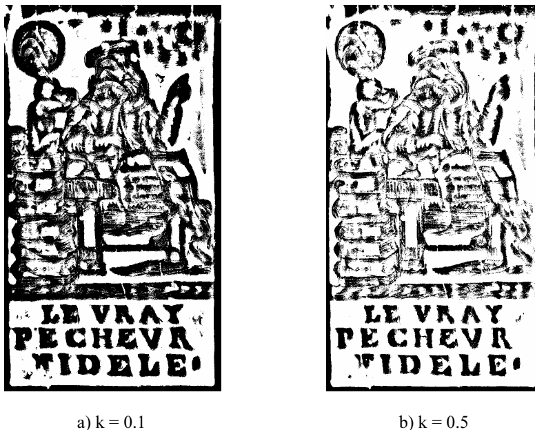
Figure 6: k effect on binarization ( t= m+ k.s )
