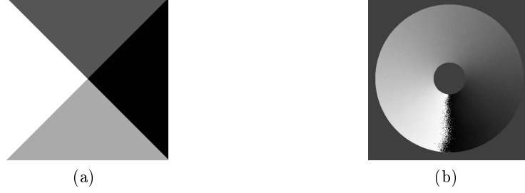
Figure 5. Disambiguation of the azimuth angle: (a) segmented image ( I_{quad} \in \{0, 1, 2, 3\} ), (b) image of the resulting azimuth angle \phi ( \phi \in [-\pi/2, 3\pi/2] ).
