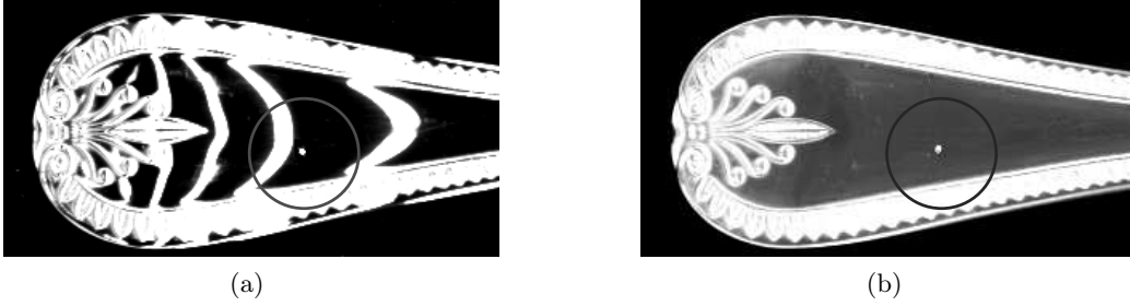
Figure 2. Defects detection with the dynamic lighting: (a) One frame of the acquisition system, and (b) Aspect image.
