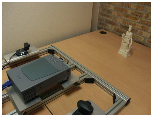
Figure 2. System composed of two cameras and one projector
