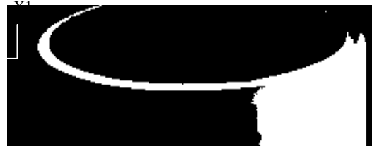
Fig 14: Binary image obtained after the threshold procedure
