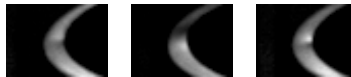
Fig 12: Different examples of defects located on the top part of the tube and revealed thanks to the low angle lighting system.
