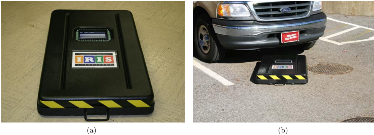
Figure 3. These images depict the first prototype for the SAFER Mobile Sensor Platform. (a) The configurable sensor bay has a view portal just above the IRIS logo in this image. (b) The low-profile platform can navigate remotely under vehicles.
