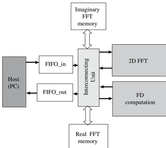
Fig. 8 Data-flow architecture of the hardware accelerator
