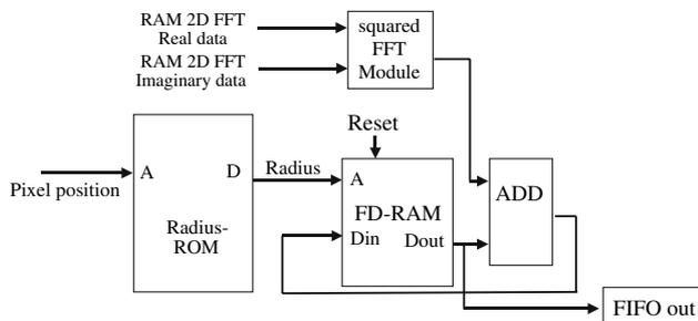
**Fig. 11** Block diagram architecture for computing Fourier Descriptors
