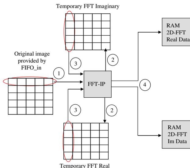
Fig. 9 Diagram block of 2D-FFT computation
