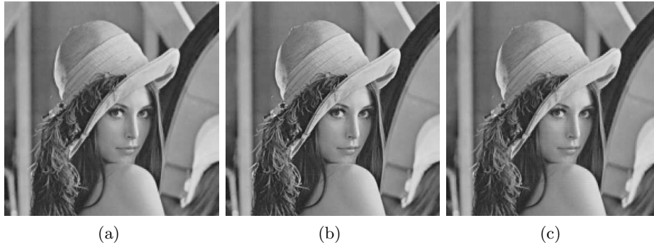
Figure 8. Reconstructions of Lena at around 55% compression rate, using: (a) tilage definition, (b) mean value simplification and (c) simplification by linearity.
