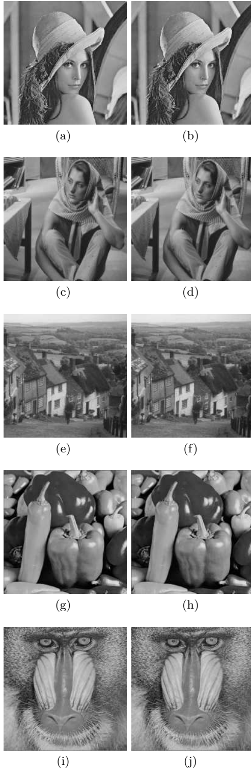
Fig. 10. Reconstruction of (a)(b) lena, (c)(d) barbara, (e)(f) goldhill, (g)(h) peppers and (i)(j) mandrill, using about 50% and 80% (respectively) of the number of original image pixels.
