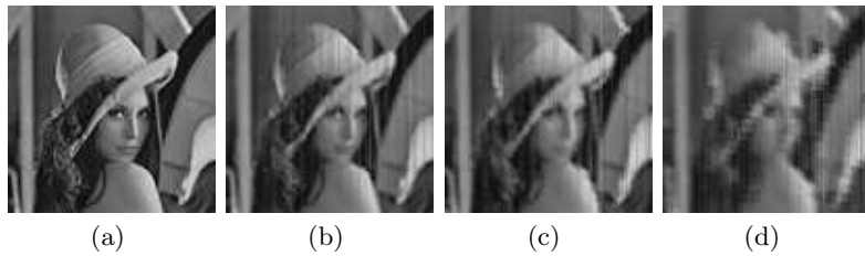
Fig. 6. Lena reconstruction, using 100%(a), 70%(b), 40%(c), 15%(d) of original image pixels.
