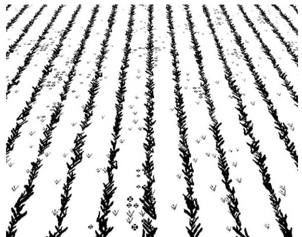
Fig. 2. Picture of a virtual field through an optical system. The simulation parameters are summarized in Table 1 for a wheat field with a mixture of two weed spatial distributions. The initial inter-row WIR ( iWIR_{inter} ) is 15.28%.
