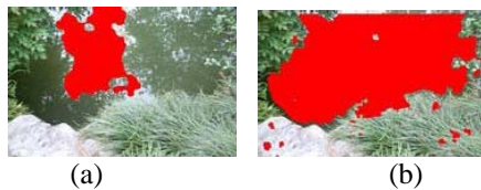
Figure 6. Water segmentation by polarization degree (left) and by Polarization phase(right), water detection is shown in red [8]
