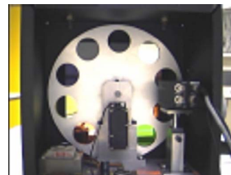
Figure 1. The multispectral system we use. It is based on monochromatic camera and a set of 10 interference filters.
